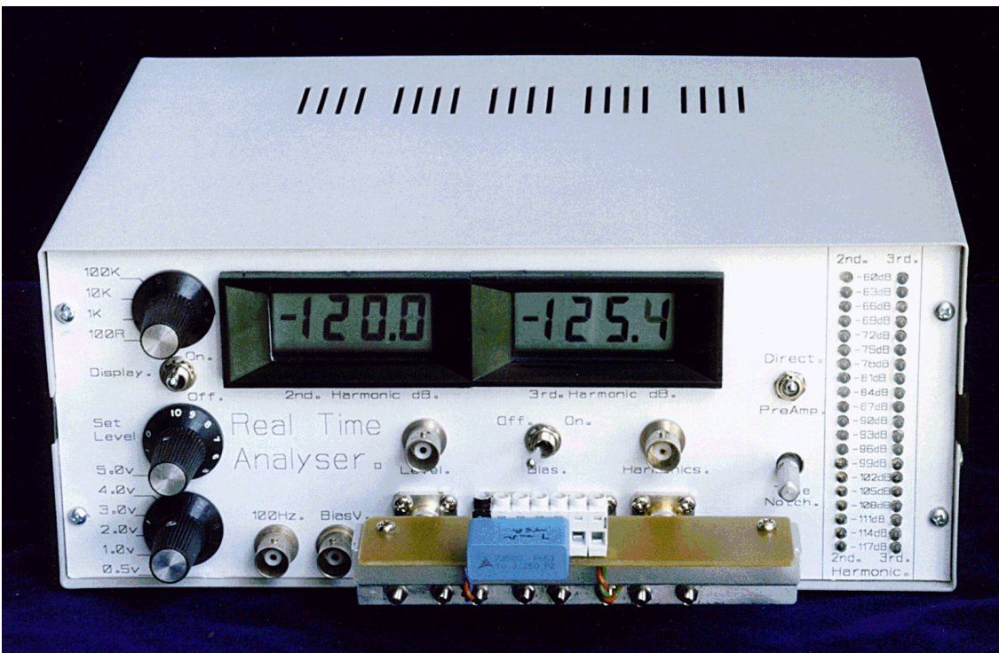
Figure 3) Testing the 1µF 250v B32653 capacitor which featured in my last article, mounted in my easily fabricated, low cost, four terminal 'replica' capacitor test jig made from a 100mm length of 15mm Aluminium angle, four panel mounting BNC connectors at 22mm centres and a terminal test strip.
