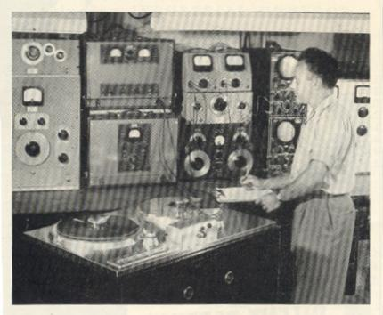
DESIGNED to fit the requirements of f-m broadcast application, the Ampex tape recorder provides a 35-minute transcribing capacity at 30 inches of tape per second. Included are precision tape drive, completely-shielded plug-in head housing with separate heads for erase, record, and playback and separate record and playback amplifiers.
