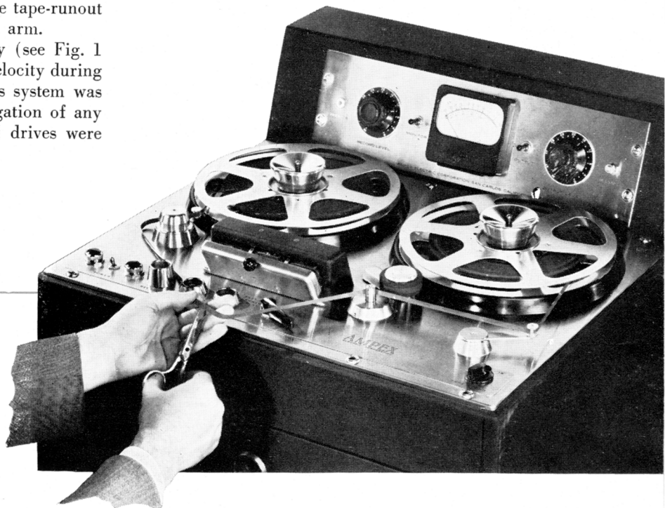
Fig. 2—Recorder in operation: Tape tension has been relaxed to facilitate tape editing, after which open gate of head
