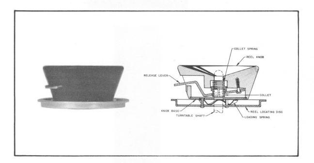
The #9093 Knob has a simple, positive action. It is slipped on the turntable shaft with the concave side facing outward, and is pressed down firmly so that the reel locating disc is engaged in the center of the reel. A spring loaded collet within the knob engages the turntable shaft. The Knob is self-centering, as the knob base is mechanically coupled to the reel locating disc through a loading spring.
