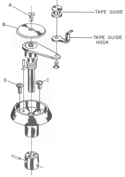
TO REMOVE ASSEMBLY FROM TOP PLATE REMOVE SCREW A, DISC B & SCREWS C & D. LIFT OUT.
