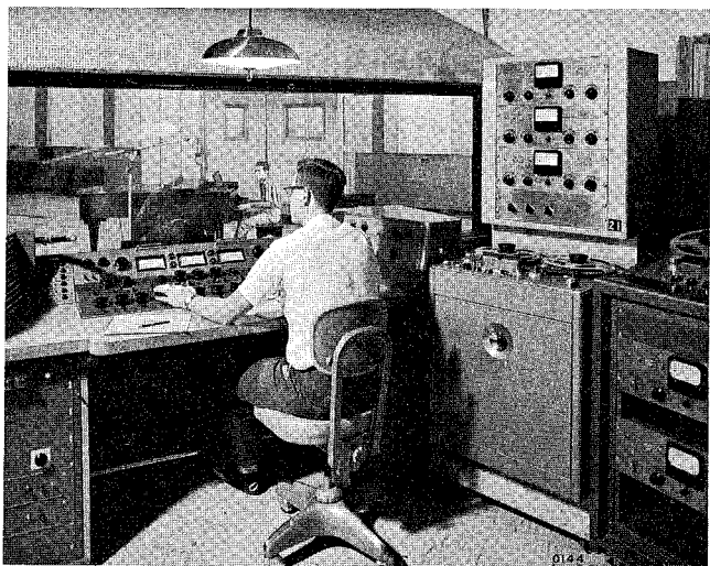
Magnetic equipment in the recording industry. Ampex Model 300-3 installed at United Recording Studios, Hollywood.
