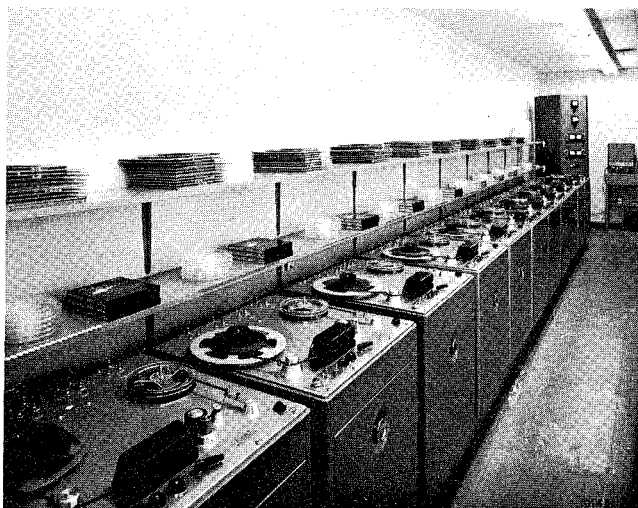
Duplicating equipment at Magnetic Tape Duplicators, Hollywood. Ampex duplicating equipment produces copies of master tapes at high speed with as many as ten copies produced with each run of the master.
