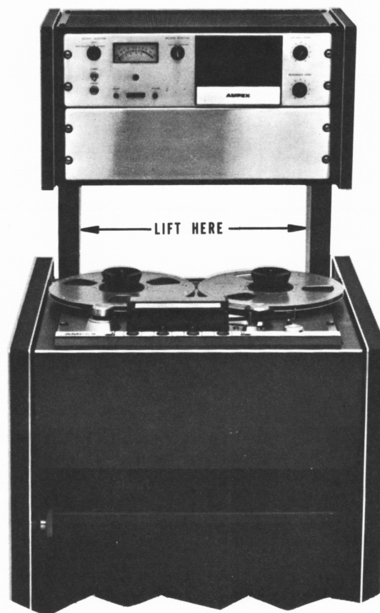
Fig. 2-1 Lift Points, Console Mounted Equipment
