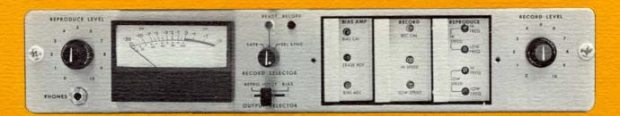
New 100% solid state plug-in modules provide the electronic sophistication to match the mechanical perfection of the new AG-440 — slim and compact. Ampex's engineering capability on the design of solid state circuitry for Digital, Instrumentation, Videofile\* and professional Videotape Recorders is reflected in the design of the AG-440 electronics.
