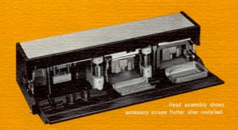
You can convert a recorder from ½ to ¼ inch operation or change track configuration in less than four minutes by removing three screws and inserting a new assembly. Registration dowel pins assure quick alignment. These are the finest, newest assemblies in Ampex's twenty year history of the manufacture of quality heads.
