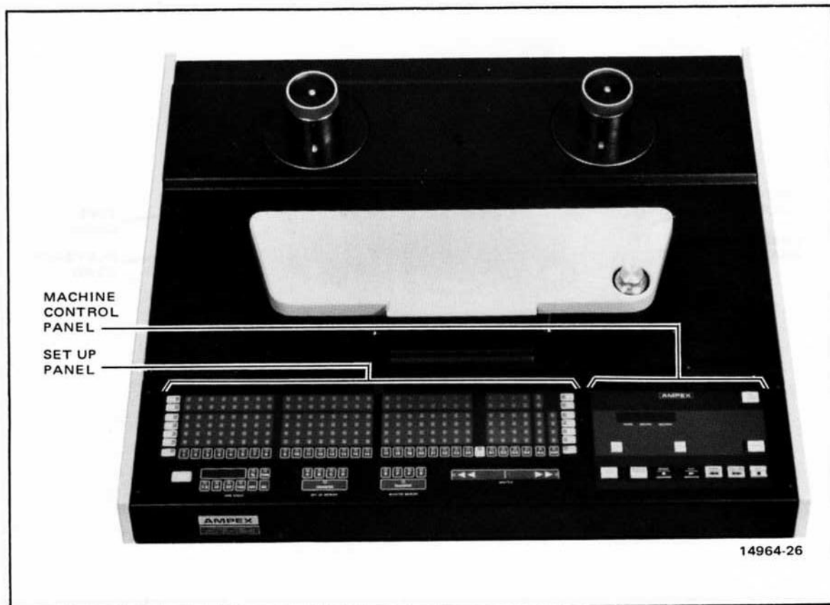
Figure 1-11. Setup and Machine Control Panels
