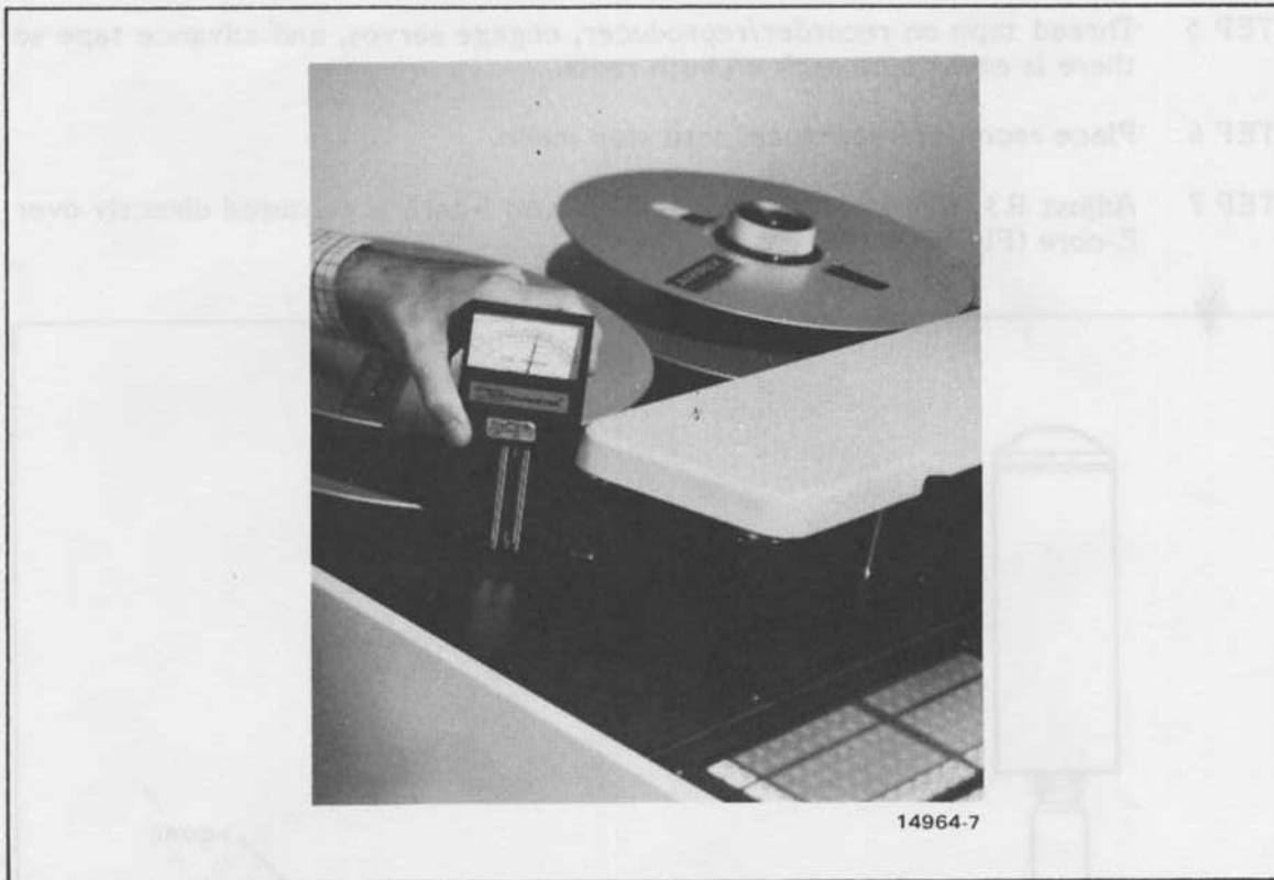
Figure 5-11. Measuring Tape Tension
