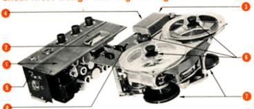
● Separate record and playback amplifiers ● Direct reading meter for both playback and recording levels ● Separate erase, record and playback heads ● Magnetic playback head gap width: .00025" ● Low impedance output ● Extremely close tolerances in all bearings and shafts ● Tape tension controlled to 8 ounces maximum ● Illuminated safety button to indicate recording mode.
