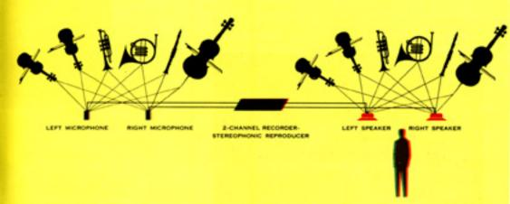
Ampex Stereophonic Sound spreads the entire orchestra out in front of you; the sound of each instrument reaches you from the same apparent source and direction "heard" by the recording microphones.
