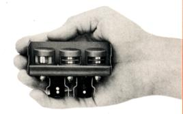
The head assembly consists of a Full-Track ERASE, Two-Track RECORD, and Two-Track PLAYBACK arrangement, in this order.
