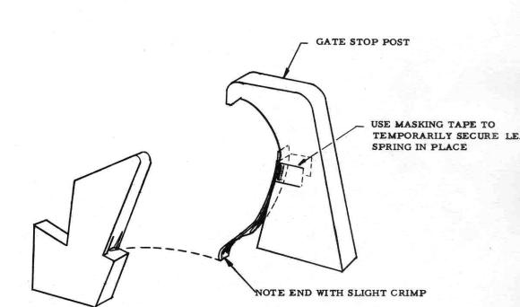
WHILE HOLDING GATE OPEN, PLACE GATE STOP POST IN POSITION AS INDICATED BY DOTTED LINE.
