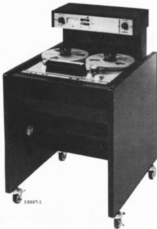
Figure 1-6. One-Channel (1/4-Inch Tape Width) Recorder/Reproducer
