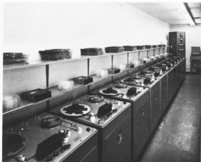
Duplicating equipment at Magnetic Tape Duplicators, Hollywood. Ampex duplicating equipment produces copies of master tapes at high speed with as many as ten copies produced with each run of the master.
