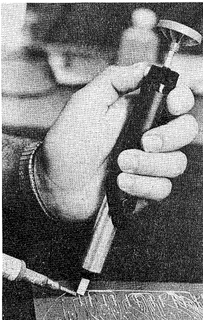
Fig. 5 Pneumatic device for removing solder.
