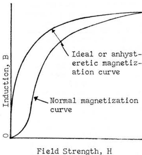
Figure 5.12 Typical Normal and Ideal Magnetization Curves
