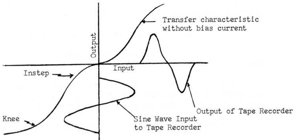
Figure 5.6 Input - Output Transfer Characteristic Without Bias
