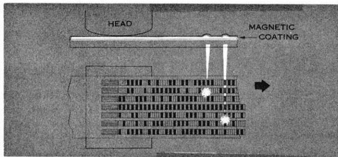
Fig. 10-5. Effect of Drop-outs in Digital Recording
