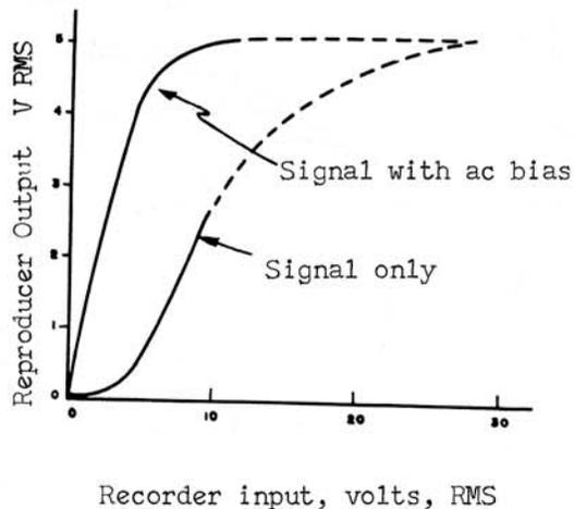
Figure 5.13 Voltage-Transfer Characteristics of a Magnetic Tape Recorder, with and without AC Bias. (3 mil Wavelength)
