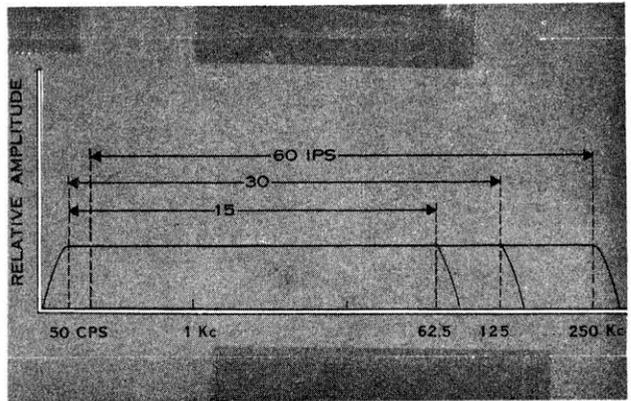
Figure 7-6. Direct-Record Frequency Response
