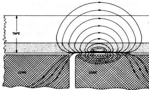
Figure 5-2 Flux Distribution of Recorded Tape in Reproducing-Head Gap Region
