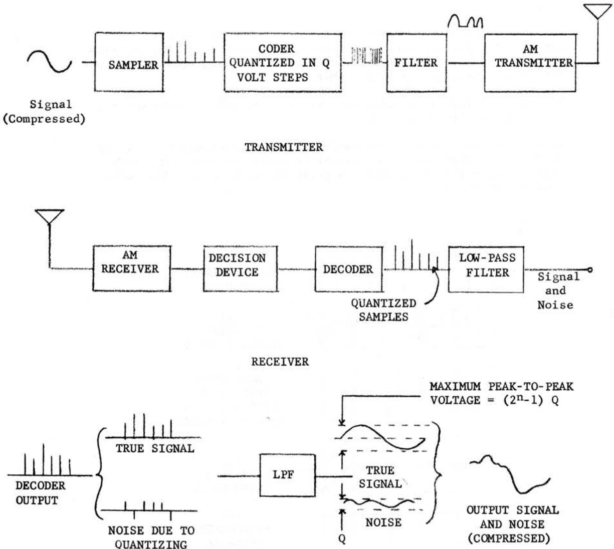
Figure 11-3 A PCM/AM System Showing Noise Due To Quantizing
