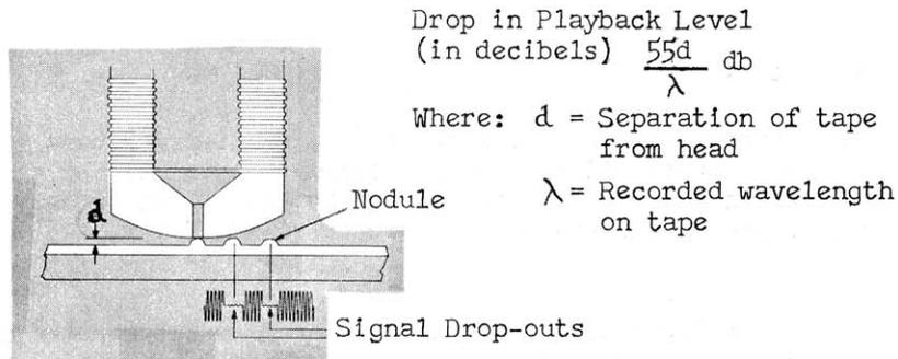
Figure 5.17 Effect of Tape-Surface Imperfections
