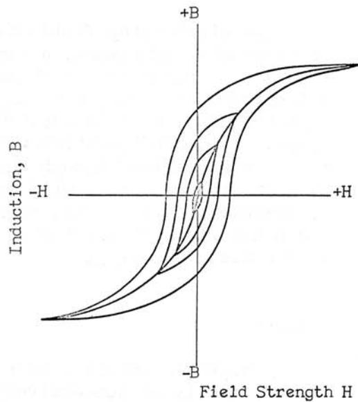
Figure 4.6 The Transduction Curve (Demagnetization)
