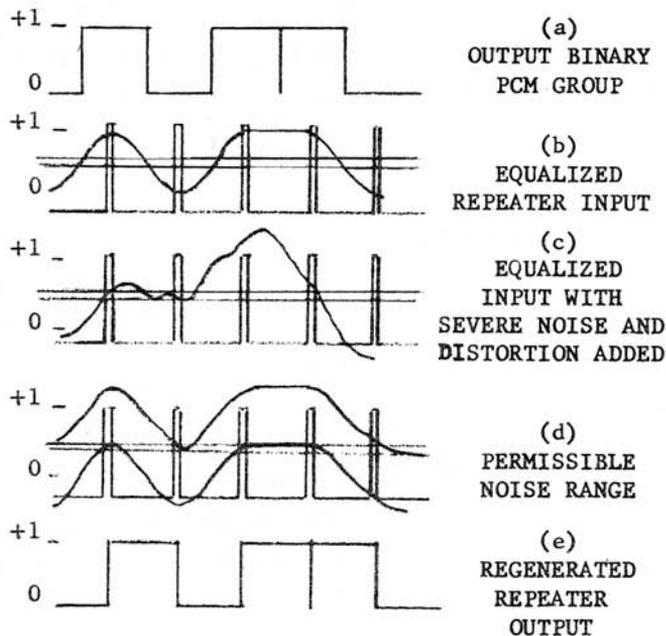
Figure 11-4 Input of a Coded Signal to a Receiver or Repeater
