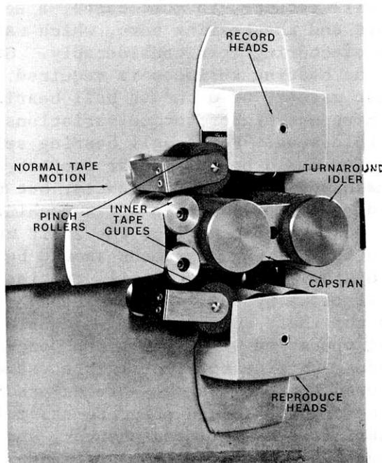
Fig. 6-5. Capstan and Pinch Roller Assembly
