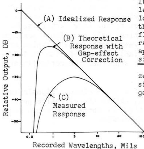
It is well known that as the wavelength approaches the effective length of the gap, the ratio of the flux linking the coil to the flux in the tape decreases. The rate of decrease is described approximately by the periodic function  $\frac{\sin x}{x}$ . This function reduces to zero when the wavelength of the signal is equal to the length of the gap.
