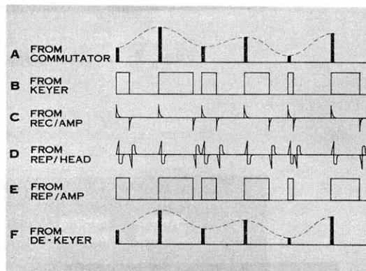
Fig. 9-6. Signals at Various Points In PDM
