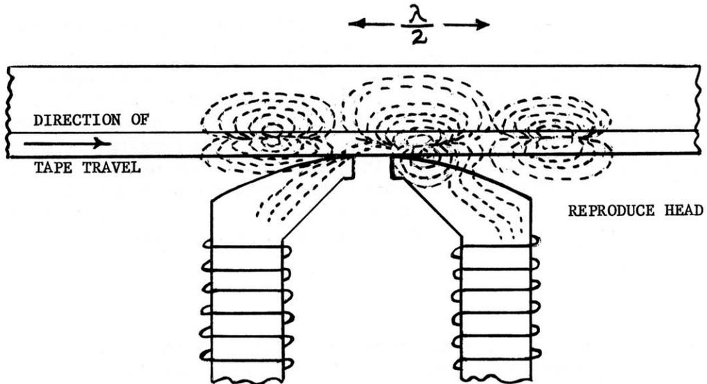
Fig. 5-16. Long Wavelength Losses
