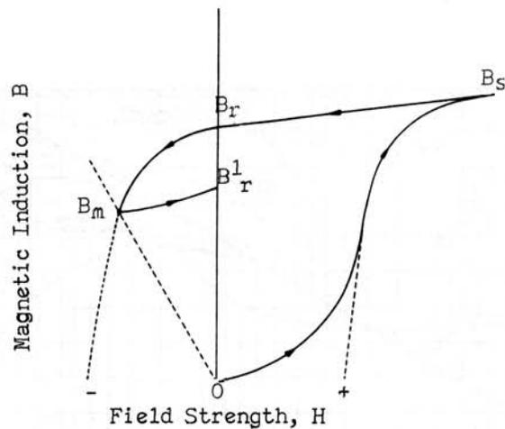
Figure 5.11 Normal Magnetization and Hysteresis Curves, Showing Demagnetization and Partial Recovery
