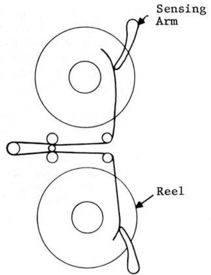
Fig. 6-13. Simple Tape Sensing System
