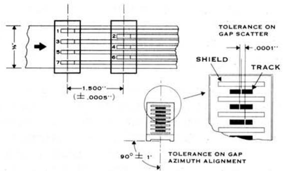
Figure 2-5. Ampex Mechanical Tolerances
