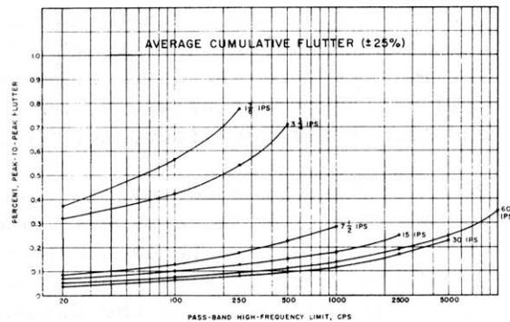
Fig. 6-7. Cumulative Flutter Curve
