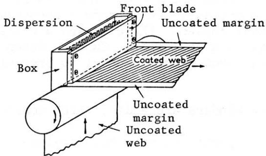
Figure 3-2. Knife Coating Process
