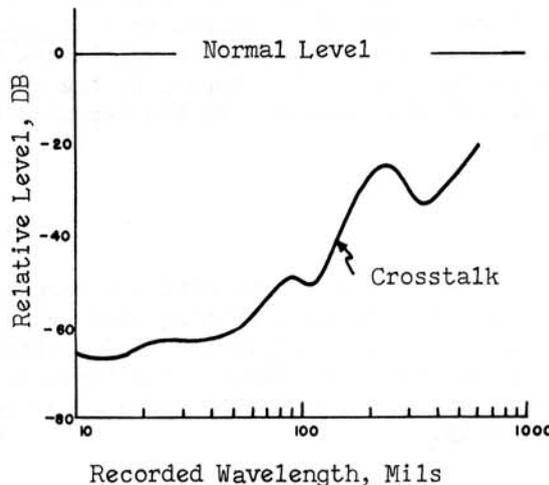
Figure 5.20 Typical Intertrack Crosstalk Between 50-Mil Tracks Spaced 70-Mils Center-to-Center
