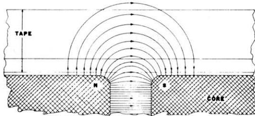
Figure 5-1 Leakage Flux Distribution in Recording-Head Gap Region
