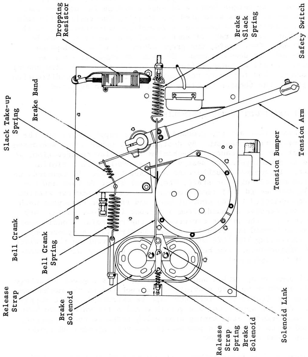
Fig. 6-16. Typical Reel Assembly With Mechanical Servo Tension Control
