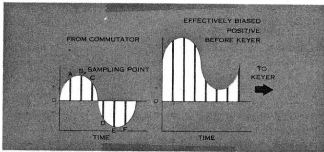
Fig. 9-1. Sampling a Signal in PDM
