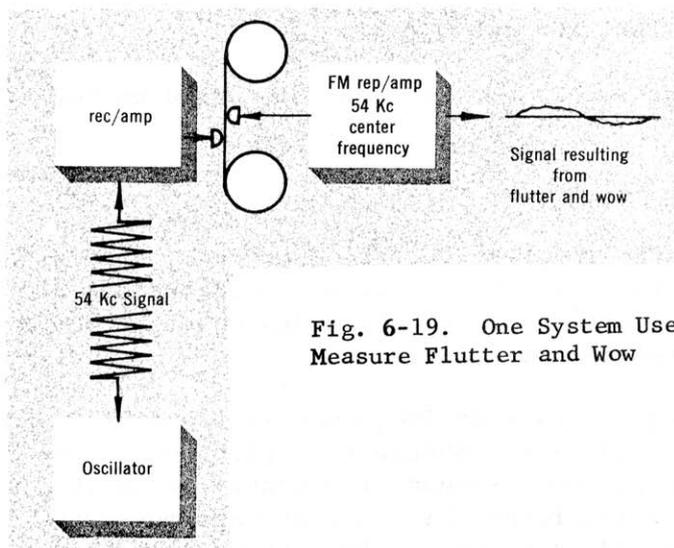
Fig. 6-19. One System Used to Measure Flutter and Wow
