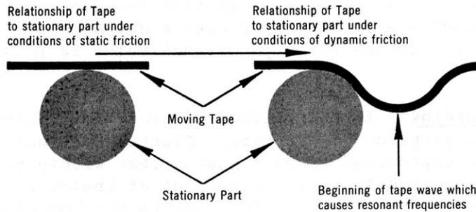
Fig. 6-18. Transition From Static to Dynamic Friction Showing Resonant Frequencies That Can be Created
