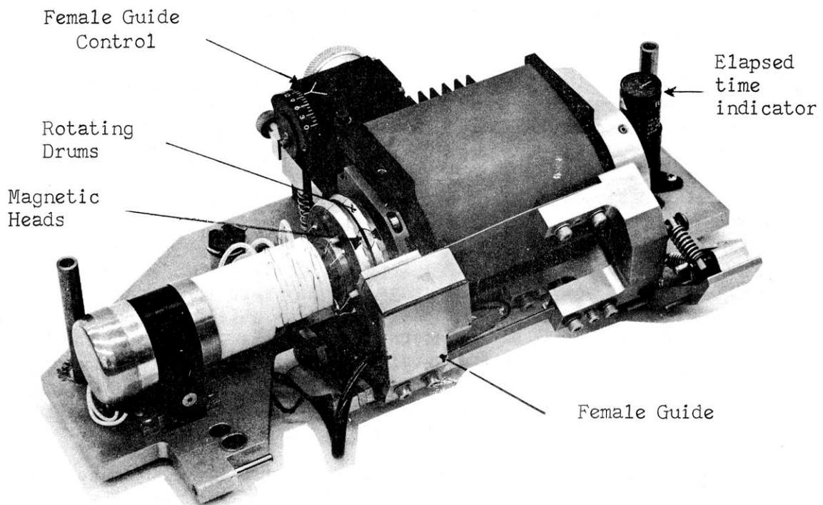
Figure 2.11 WIDEBAND ROTARY HEAD ASSEMBLY
