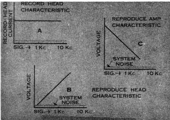
Fig. 7-3. Effect of Frequency on Recording and Reproducing Characteristics
