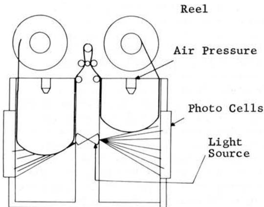
Fig. 6-12. Tape Storage Container Using Vacuum and Photoelectric Sensing
