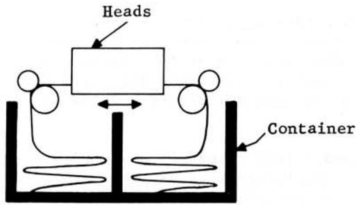
Fig. 6-10. Simple Tape Storage Container
