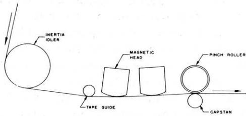
Fig. 6-1. Open-Loop Drive System
