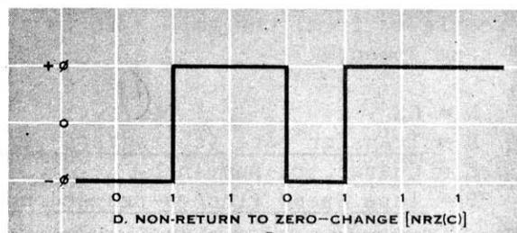
Fig. 10-3. The series 0 1 1 0 1 1 1 recorded in the five most common computer formats. The differences in these formats (explained in the text) makes it necessary to use electronic translators when feeding one format into a computer designed for another.
