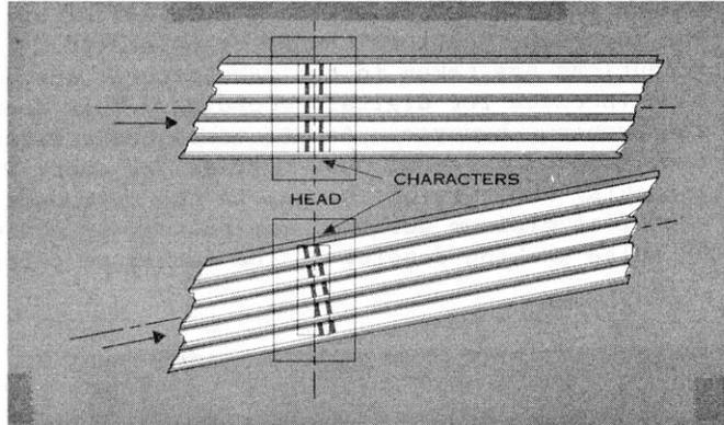
Fig. 10-6. Error Caused by Tape Skew
