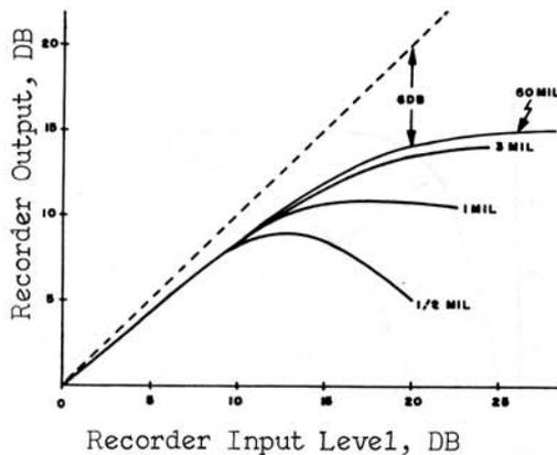
Figure 5.14 Amplitude-Transfer Characteristics of a Magnetic Tape Recorder for Four Typical Wavelengths. (Reference-Normal Level)
