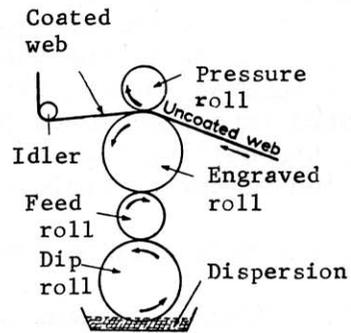
Figure 3-3. Rotogravure Coating Process
