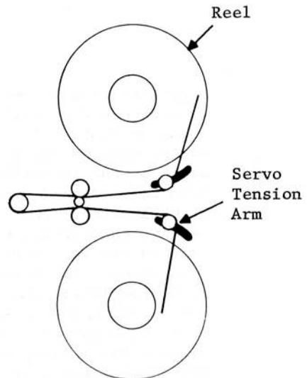
Fig. 6-14. Servo Tape Sensing System
