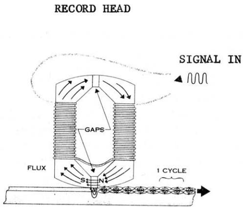
Figure 2-2 Magnetization of Tape's Oxide Particles Depends on Flux Flow in Gap at Instant Each Crosses Trailing Edge
