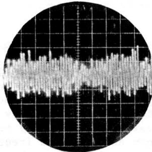
Picture of "peak-to-peak" flutter as it appears on the face of an oscilloscope. Upper spikes might represent tape speedups during playback and the consequent higher frequencies; lower spikes, speed reductions and reduced frequencies.
