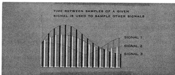
Fig. 9-2. PDM Sampling Technique
