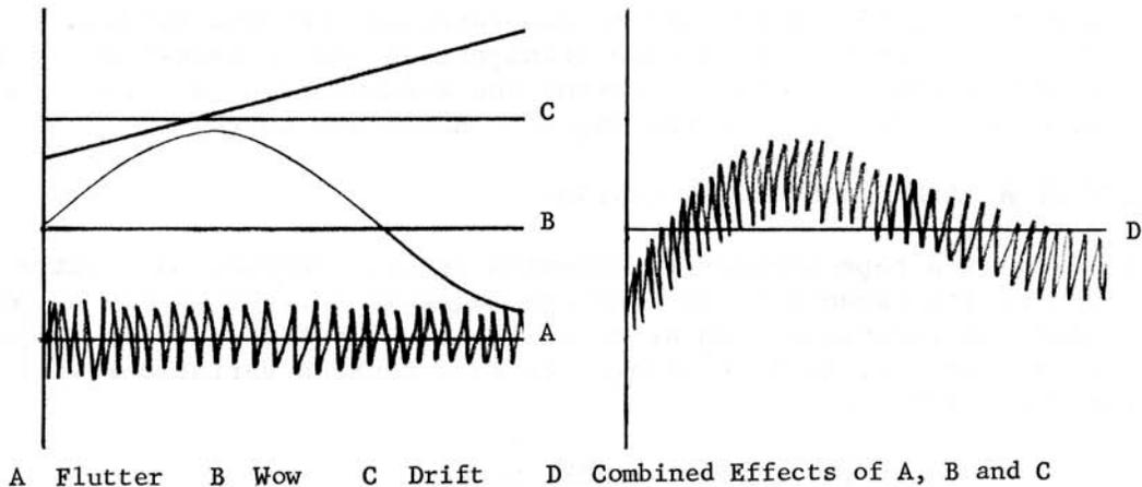
Fig. 6-17. Relationship Between Flutter, Wow and Drift
