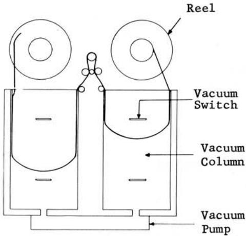
Fig. 6-11. Tape Storage Container Using Vacuum
