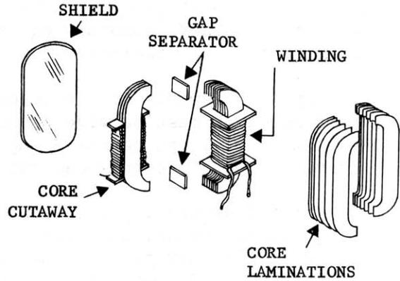
Figure 2-1 Construction and Component Parts of Magnetic Head
