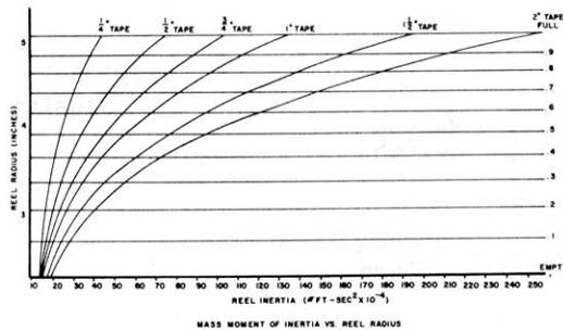
Fig. 6-15. Mass Moment of Inertia vs. Reel Radius
