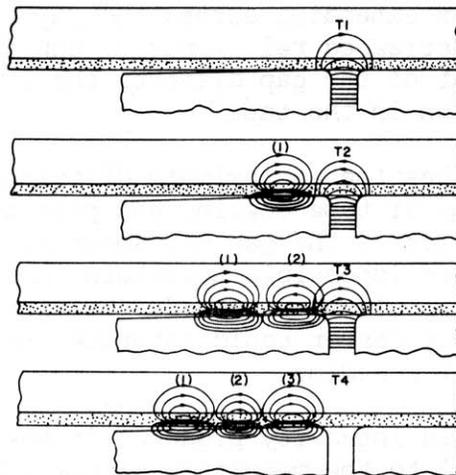
Figure 5-3 Simplified Synthesis of Recording Process
