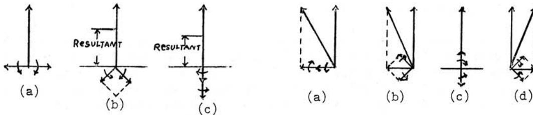
Amplitude Modulation Vector Diagrams
