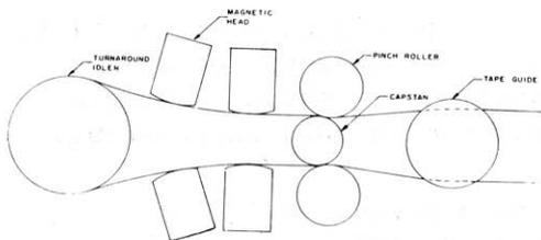
Fig. 6-3. Closed-Loop Tape Drive System
