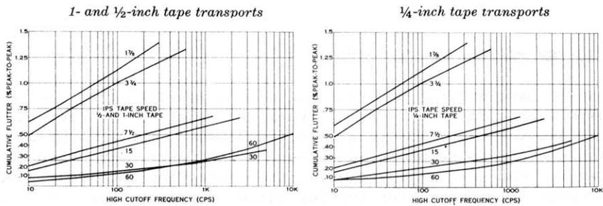
These graphs show maximum cumulative flutter as exhibited by any tape-width or reel-size transport of the FR-100A series. These figures are the usual conservative specifications provided for Ampex equipment, and were purposely not made from selected or peaked-up units.
