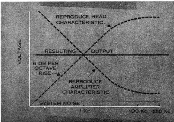
Fig. 7-4. Reproduce Amplifier Output
