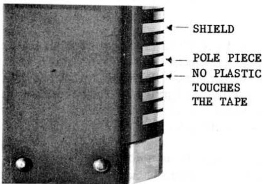
Figure 2-8. Head Surfaces Isolated in Newest Design
