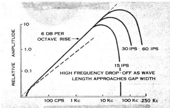
Fig. 7-5. Reproduce Head Output
