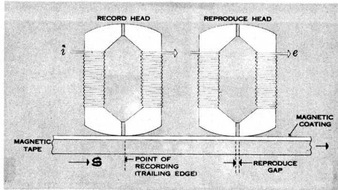
Fig. 7-2. The magnetic tape recording and reproducing process
