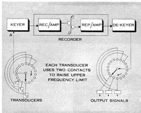
Fig. 9-5. PDM Recording
