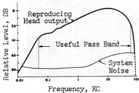
Figure 5.19 Unequalized System Noise and Reproducing-Head Output vs Frequency. Normal-Level, Constant-Current Recording at 30 IPS
