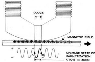
Figure 2-4. Effect of Wave Length and Gap Size on Reproduction Output
