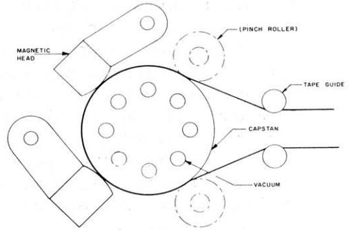
Fig. 6-2. Zero-Loop Tape Drive System
