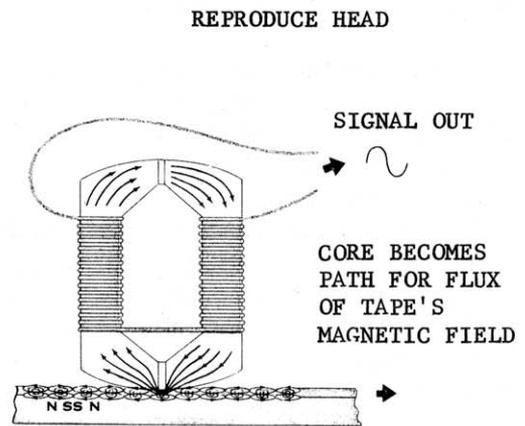
Figure 2-3 Reproduction of Signal From Magnetic Tape
