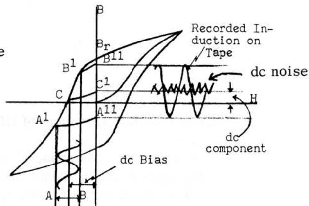
Figure 5.8 Alternate Method of Applying DC Bias. Tape Pre-magnetized to Saturation before Signal Applied with DC Bias.
