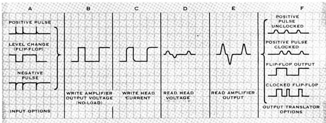
Fig. 10-4. Signal Waveshapes From Input to Output Through Ampex Digital Electronics
