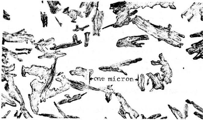
Figure 3-1. Sketch of Electron Microscope Presentation of Magnetic Oxide Particles, Showing Typical Size and Shape.
