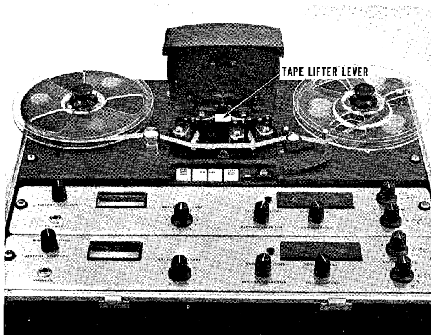
Fig. 3-3. Tape Threading Path and Tape Lift Lever
