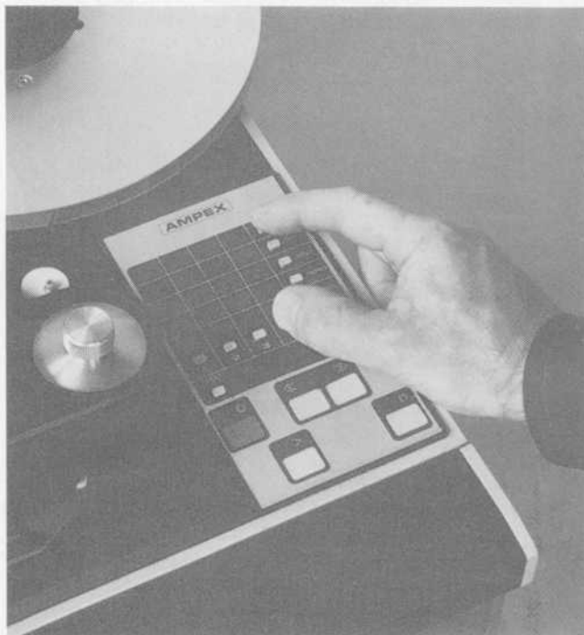
A closeup of the ATR-100 control panel matrix.
