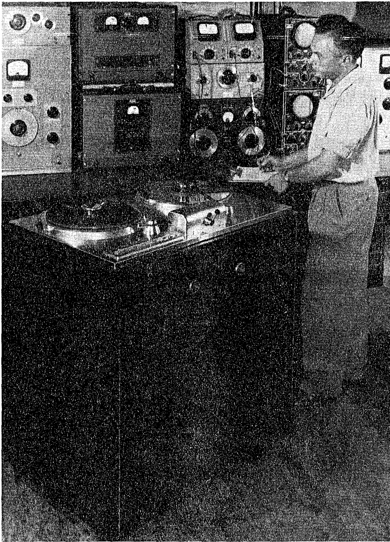
THE AMPEX MODEL 200, the magnetic tape recorder developed by Harold Lindsay in the late 1940s, revolutionized the recording industry.
