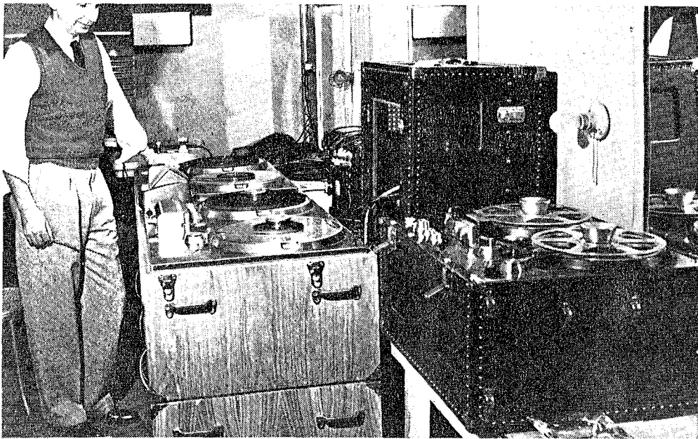
Mullin in 1950 with two "portable" Model 200 Ampex tape recorders (note the handles) and the first Model 300 to leave the factory. With these three machines, Mullin had available a full range of advanced editing techniques.
