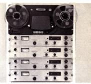
AL-500-4; a four channel, four track recorder/reproducer with speeds of 15/16 and 17/8 ips. The AL-500 records four tracks simultaneously, or by switching, can record 1 or more tracks from single or multiple source, Maximum continuous recording time is 8 hours and 32 minutes in one direction using 1/2 mil tape on 7" reel.
