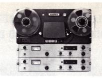
AL-500-2; a two channel, four track recorder/reproducer operating at selectable speeds of  $^1\%_6$  and 1% ips. Tracks 1 and 3 are recorded on the first pass; tracks 2 and 4 on the second by transposing the reels. The AL-500 will accept two simultaneous incoming signals, or can be switched to record one track at a time, giving a total of 34 hours - 8 minutes on a single 7" reel of 1/2 mil tape.
