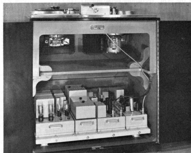
Front view with cabinet doors opened. Note modular electronic assembly on vibration-isolated base. Removable modules are (left to right) power supply, control logic assembly, record module, and playback module.
