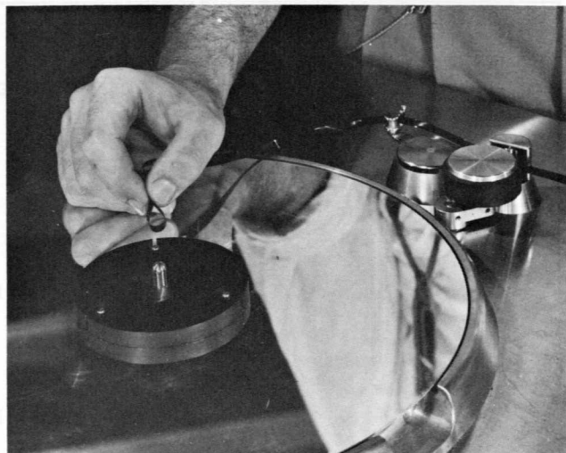
Threading the 14"-diameter open-faced "reel." Reel held 5400 ft. 0.002" thick tape. Torque/threading pin mounting circle dimensions have carried over to present day N.A.B. Standard Hubs as inside (hub bore) driving slots.
