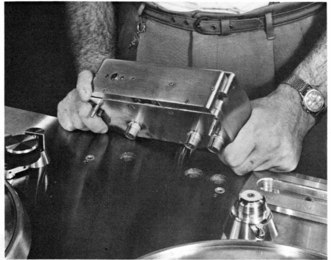
View illustrating plug-in feature of magnetic head assembly. Slotted cap screw at left of head gate covers hole for editing pencil insertion over playback gap.
