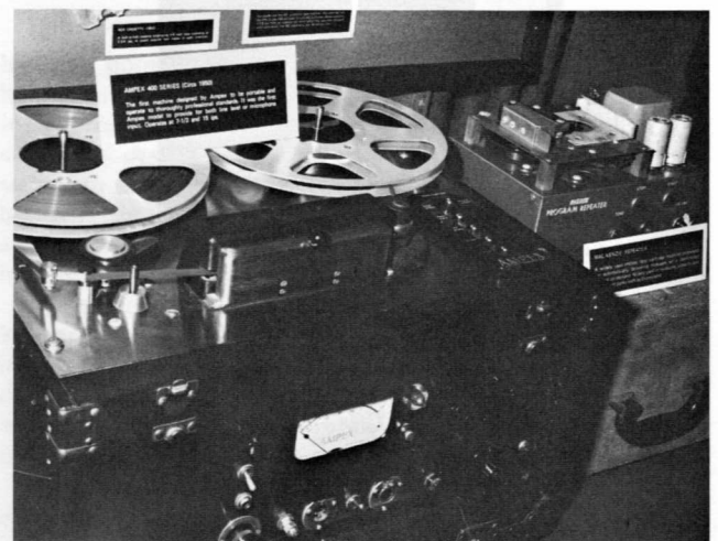
A new model appeared in 1950. This is an Ampex 400, the first portable machine designed to professional standards. It was also the first machine to provide for both the level and microphone input. It operates at 7.5 or 15 in./sec. speed. Photo from Jack Mullin's product museum as shown at a recent AES Convention.
